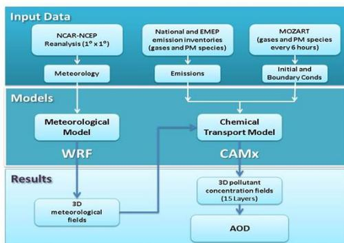
Figure 1. Air quality modelling system – input/output structure
