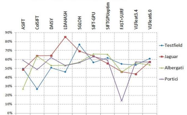
Figure 5: The visibility of the derived 3D points in more than 3 images (normalized with respect to the all extracted points).
