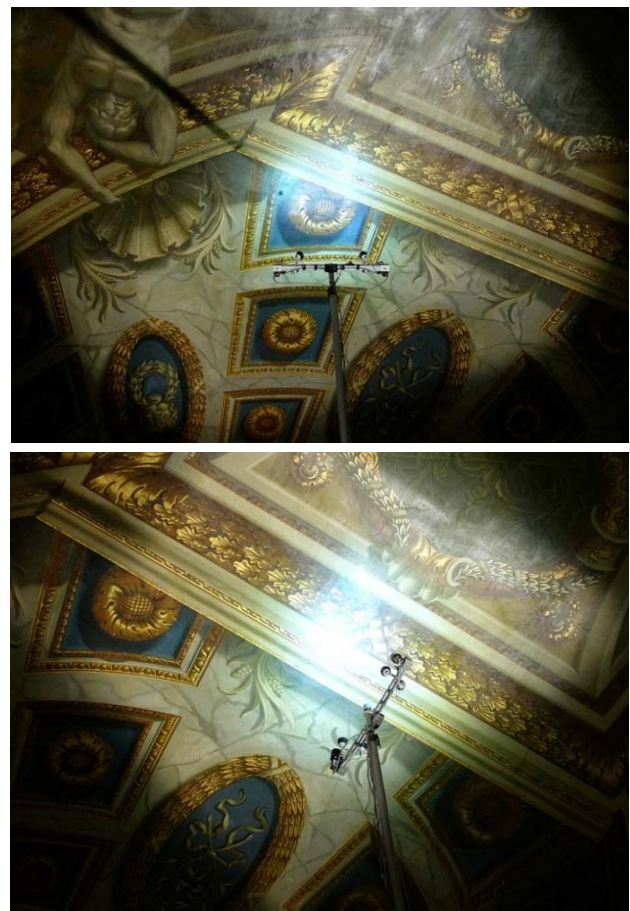
Figure 6. Mast deployed at two locations, showing the circle of yellowish light on the ceiling from floor-mounted spotlights and the localised bluish illumination from the four LED lights on the mast head.
