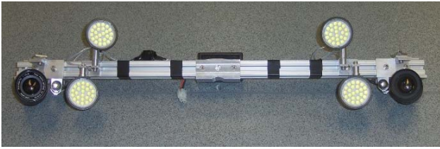
Figure 3. Top view of the camera rig, showing camera lenses, positioning lasers and LED lights.
