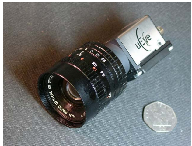
Figure 2. Miniature uEye camera fitted with Fujinon 9mm C-mount lens. The 50p coin shows the relative size.
