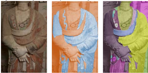
(a) Original Image (b)GrabCut (c)Watershed Figure 1. Texture image segmentations is acquired with GrabCut and Watershed algorithms.
