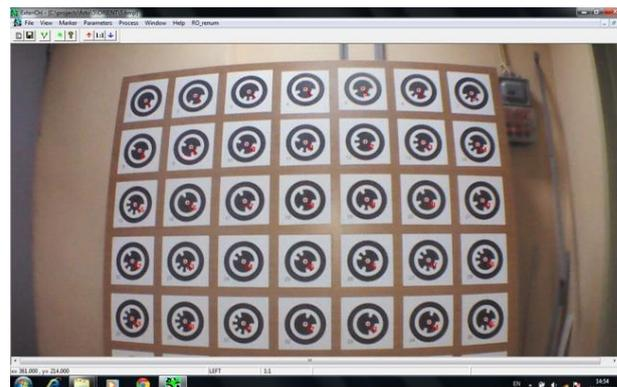
Figure 6. The test field image acquired by frontal camera.
