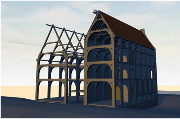
Figure 3. Reconstruction of the timber frame (image by L. Opgenhaffen)
