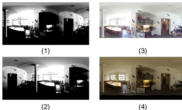
Figure 4: Image-based registration: the normalized panoramic image taken with the DSLR (2) has to be aligned to the normalized panoramic image which was exported from the laser scanning unit (1). The automatic alignment described in Section 4.2 produces an aligned high-resolution panoramic image (4) which is aligned to the panoramic image from the laser scanning unit (3).
