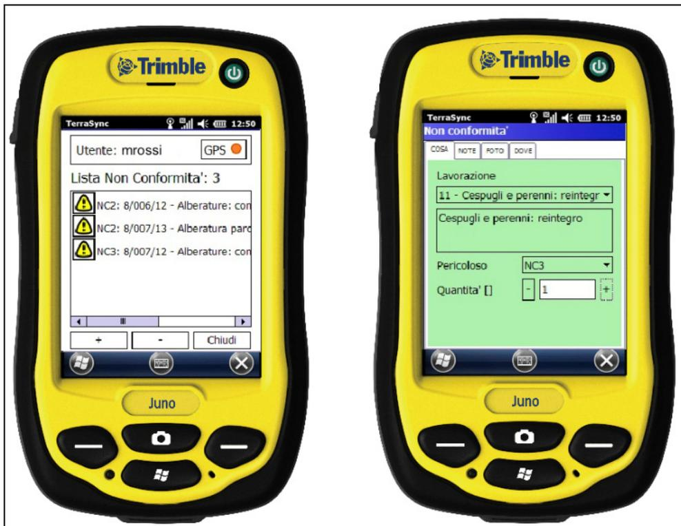
Picture 3 – Handheld device “Trimble JUNO” customized with the dissimilarity reporting software
