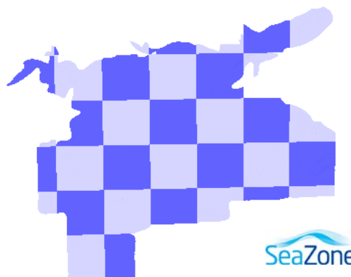
Figure 5: An example of the pattern of a tiled approximation where each tile represents one surface.
