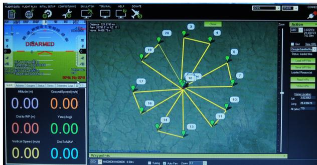
Figure 3. Rosette flight plan designed on Mission Planner©
