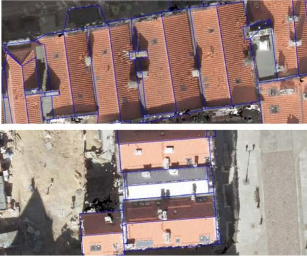
Figure 3. Examples of automatically generated 3D models of buildings with true-ortho from aerial images in a background.
