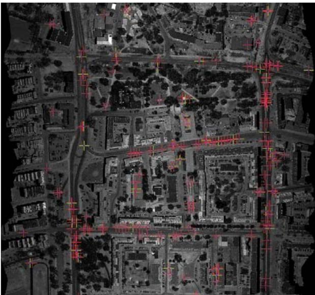
Figure 2. Spatial distribution of points measured on intensity image and true-ortho.
