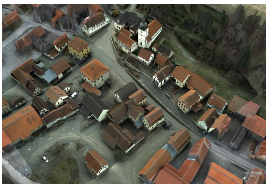
Figure 11. Texturised surface model by using vertical and oblique image data
