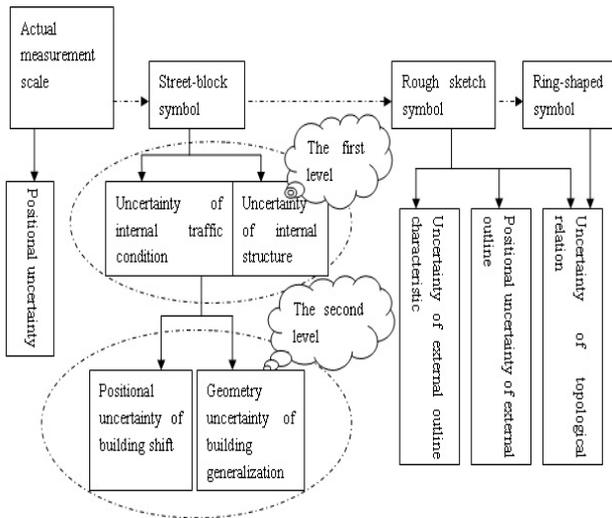
Figure 4. Uncertainty types of multi-scale representation of settlement on each scale stage
