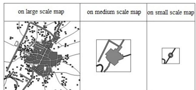
Figure 1. Graphic symbol of multi-scale representation of street-block settlement(G.R. Zhu, L.Z. Guo, etc., 2010)
