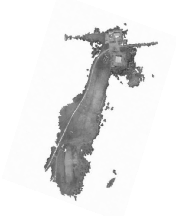
Figure 6. Dense point cloud created by VisualSFM, CMVS and PMVS from multiple flights over part of the northern test areas using the NGA quadcopter with a GoPro flat lens camera
