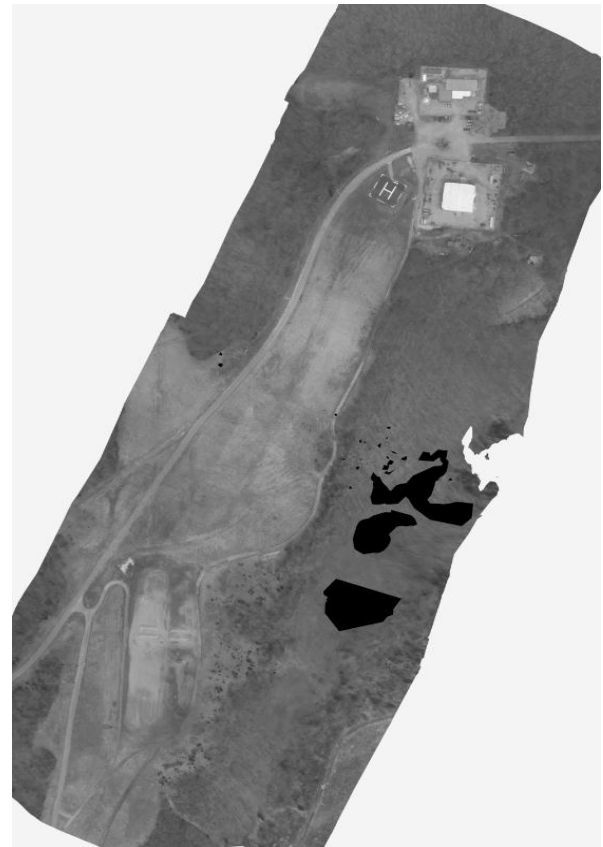
Figure 11. Orthophoto mosaic made by CMP-MVS from a NGA quadcopter with a flat lens GoPro camera
