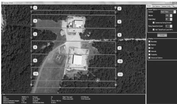
Figure 1. Mission Planner survey tool plots flight lines base on mission constraints using ©2014 Google Earth image
