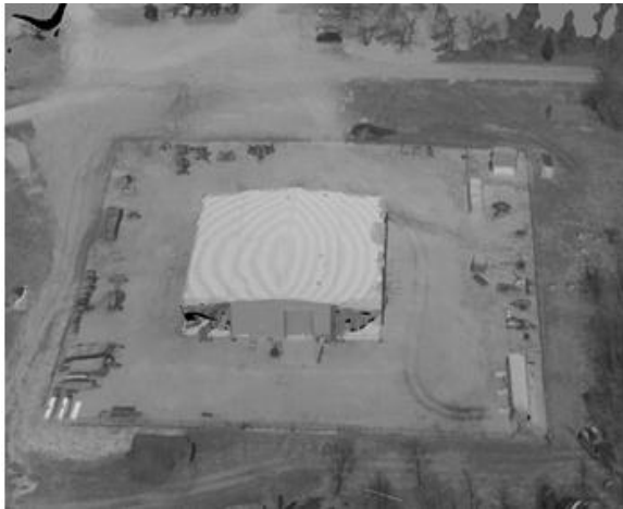
Figure 9. Textured 3D model created by Agisoft PhotoScan from single circular flight over machine storage area using the NGA quadcopter with a GoPro flat lens camera
