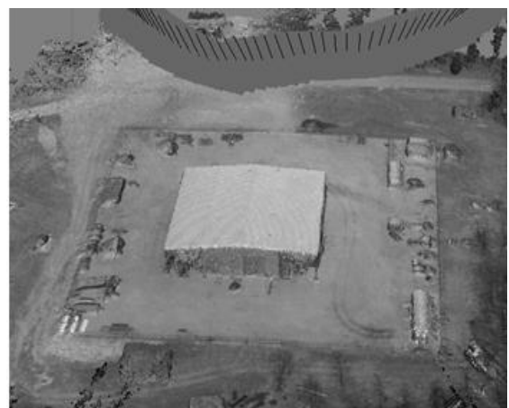
Figure 8. Dense point cloud created by Agisoft PhotoScan from single circular flight over machine storage area using the NGA quadcopter with a GoPro flat lens camera
