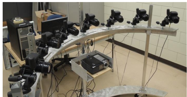
Figure 3. Multi-camera photogrammetric system consisting of seven DSLRs attached to a metal frame
