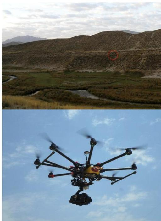
Figure 2. S1000 multirotor with Canon 5D MarkIII
