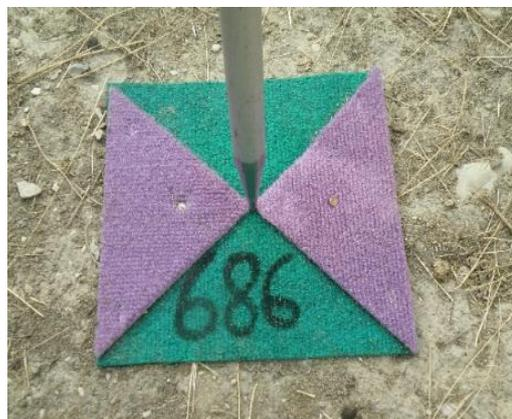
Figure 3. Artificial Ground Control Points Marker
