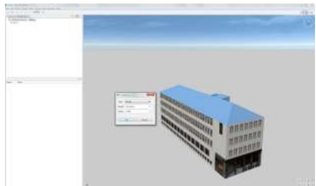
Figure 4. Illustrates the Stuttgart HFT building in LOD2 in CityServer3D (15,891 bytes in CityGML format) with the hipped roof type external code list as 1040 which is defined for Germany.
