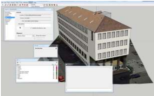
Figure 5. Illustrates HFT4 in Stuttgart which is generated automatically via Ruby programming in SketchUp Trimble.
