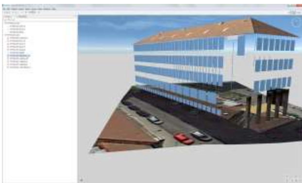
Figure 6. Illustrates HFT4 in Stuttgart in CityServer3D in LoD3 and LoD2 (1,482,276 bytes in LoD3). Some layers became invisible in CityServer3D.
