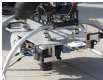
Figure 1 Damping parts of Lidar on a 100kg gasoline helicopter
