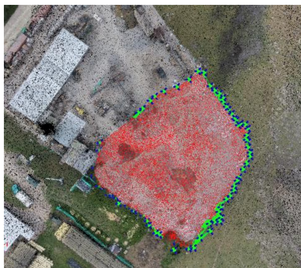
Figure 4. UAV Point cloud with stockpile drawing top view
