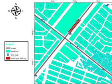
Figure. 9 An image showing the result from the system analysis in order to determine the distance the user traverses on foot to the selected station
