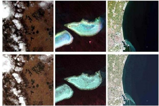
Figure (18): a new algorithm to correct the vertical noise (pictured below) with unmodified and raw image (pictured above) in CHRIS sensor images BR-2005-07-17 (pictured left), EL-2006-01-30 (middle image), PC-2005-05-18 (pictured right)
