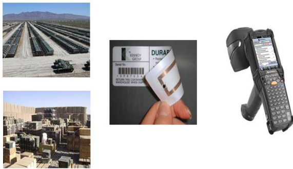
Figure 1. Connecting RFID tags to all military logistics (supplies) in all garrisons in order to control incoming and outgoing logistics via readers.
