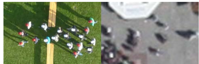
Figure 3. Comparison of an image from the UAV Falcon 8 and an image from the airborne 3K camera system: Representation of pedestrians.
