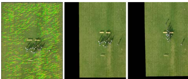
Figure 2. Coregistration example. Left: Inliers of SIFT correspondences after RANSAC procedure. Right: Reference image and aligned image in bounding boxes.
