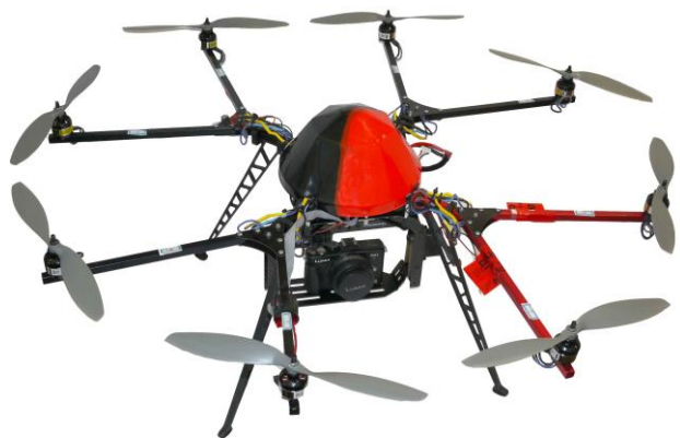
Figure 3. MK-Okto by Hisystems GmbH mounted with Lumix DMC GF3 consumer camera.
