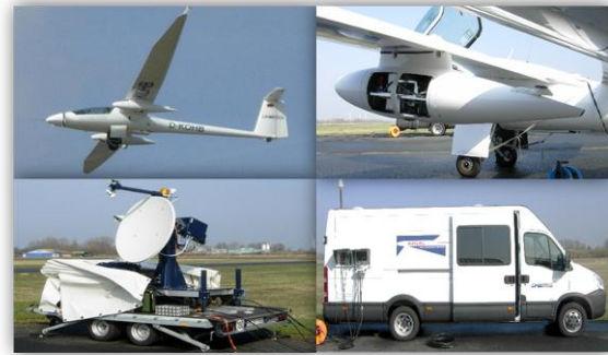
Figure 2: SELSAS-HyM Components - UL: Glider Condor, UR: Wing pod with recording unit, LL: data receiving antenna, LR: mobile ground control station
