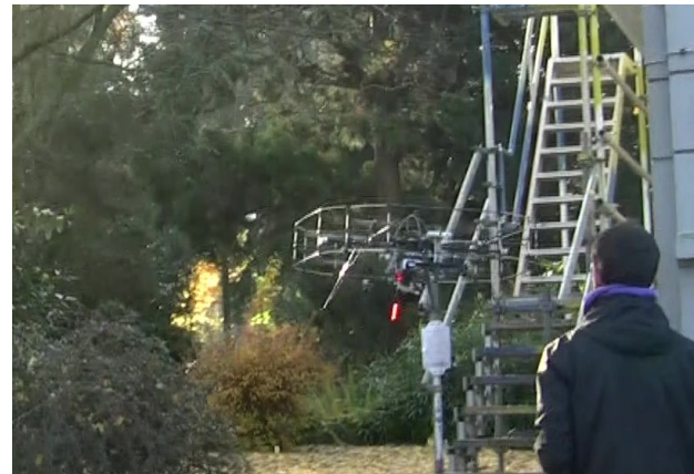
Figure 1: Our local obstacle avoidance algorithm acts as a safety measure between control inputs given by a planning layer or a human pilot remotely controlling the robot. This ensures safe operation in challenging situations, e. g., narrow passageways.
