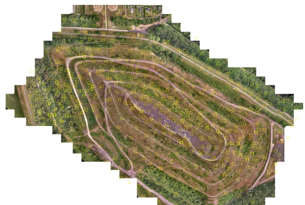
Figure 9. Tie-points in second aerotriangulation (Socet Set)
