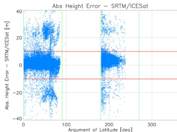
Figure 4: Height error monitoring and detection of outliers
