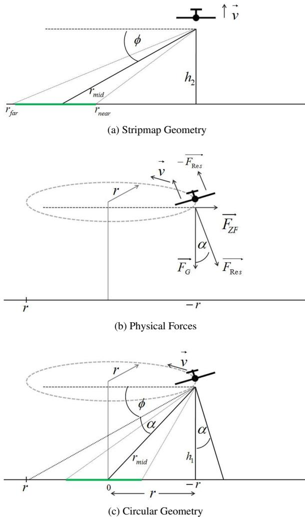
Figure 1: SAR Geometry
