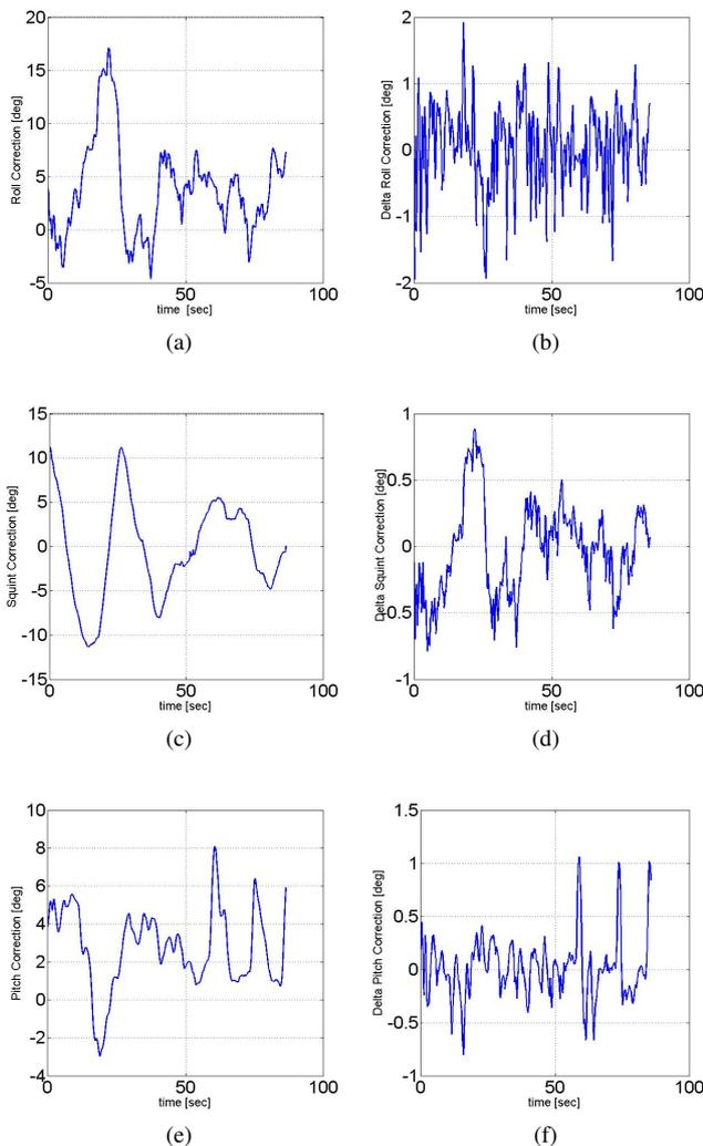
Figure 6: Stabilization Parameters for roll (a,b), squint (c,d) and pitch (e,f) showing experimental data. Total rate of correction over full trajectory on the left side - total compensation rate on the right side.
