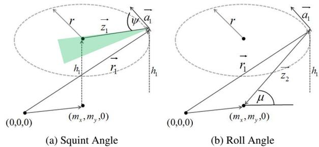
Figure 4: Calculation of optimal roll and squint angle
