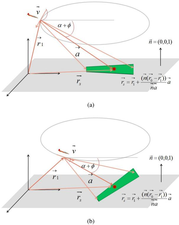
Figure 3: Circular SAR Geometry - Calculation of the instantaneous beam focus center
