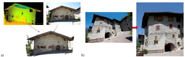
Figure 12: Range and image data co-registered to create an orthophoto of the façade (a). Produced orthophoto and vectorialization of architectural information (b).
