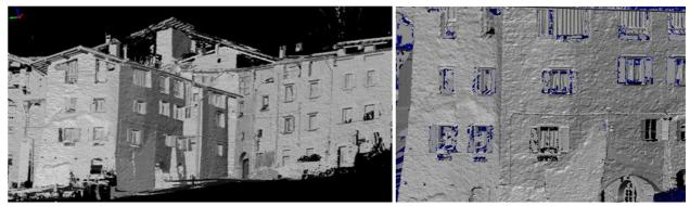
Figure 11: Some 3D results for the Calvola village. For such complex structure, the hole filling procedure is the most time consuming part of the 3D modeling pipeline.
