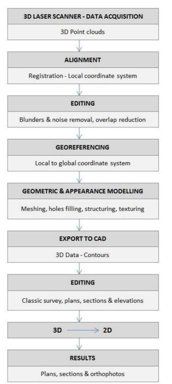
Figure 16: The flowchart of the methodology followed for the 3D surveying of complex heritages and the delivering of 2D results.
