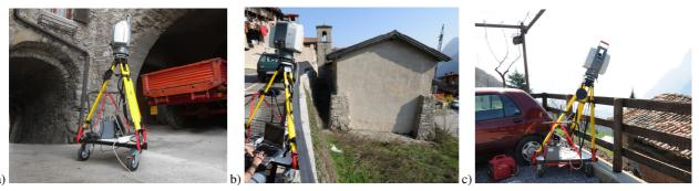
Figure 10: The laser scanner on the home-built trolley (a). Not-accessible areas which required to place the surveying instrument is difficult positions (b, c).
