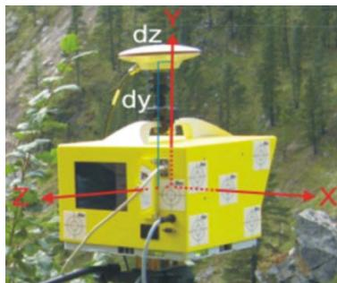
Figure 4. GPS receiver with the ILRIS GPS mount kit set placed on the scanner. Scanner reference system and offsets ( $dy$ ,  $dz$ ) between antenna phase center and scanner origin are represented.
