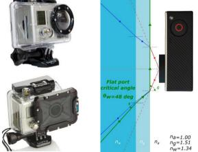
Figure 2. GOPRO HERO dome and flat ports. An early underwater housing with dome port for GOPRO HERO 1 and 2 cameras (left-up). An optional flat port replacement housing for GOPRO HERO 1 and 2 (left-down). A schematic view of the reduced field of view because of flat port critical angle (right).
