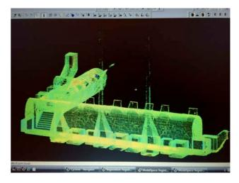
Figure 10. Three-dimensional model of the vault complex. The model was built by composing the sets of data collected with the scanner laser along the field work. Upper and lower main spaces can be clearly seen, as well as the inner stair and the wall-embedded access stair.
