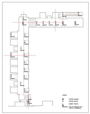
Figure 9. Location of the scanner-laser inside the cellars.
