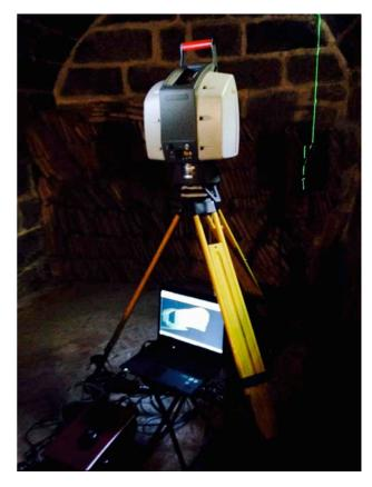
Figure 8. The laser scanner surveying the upper spaces.
