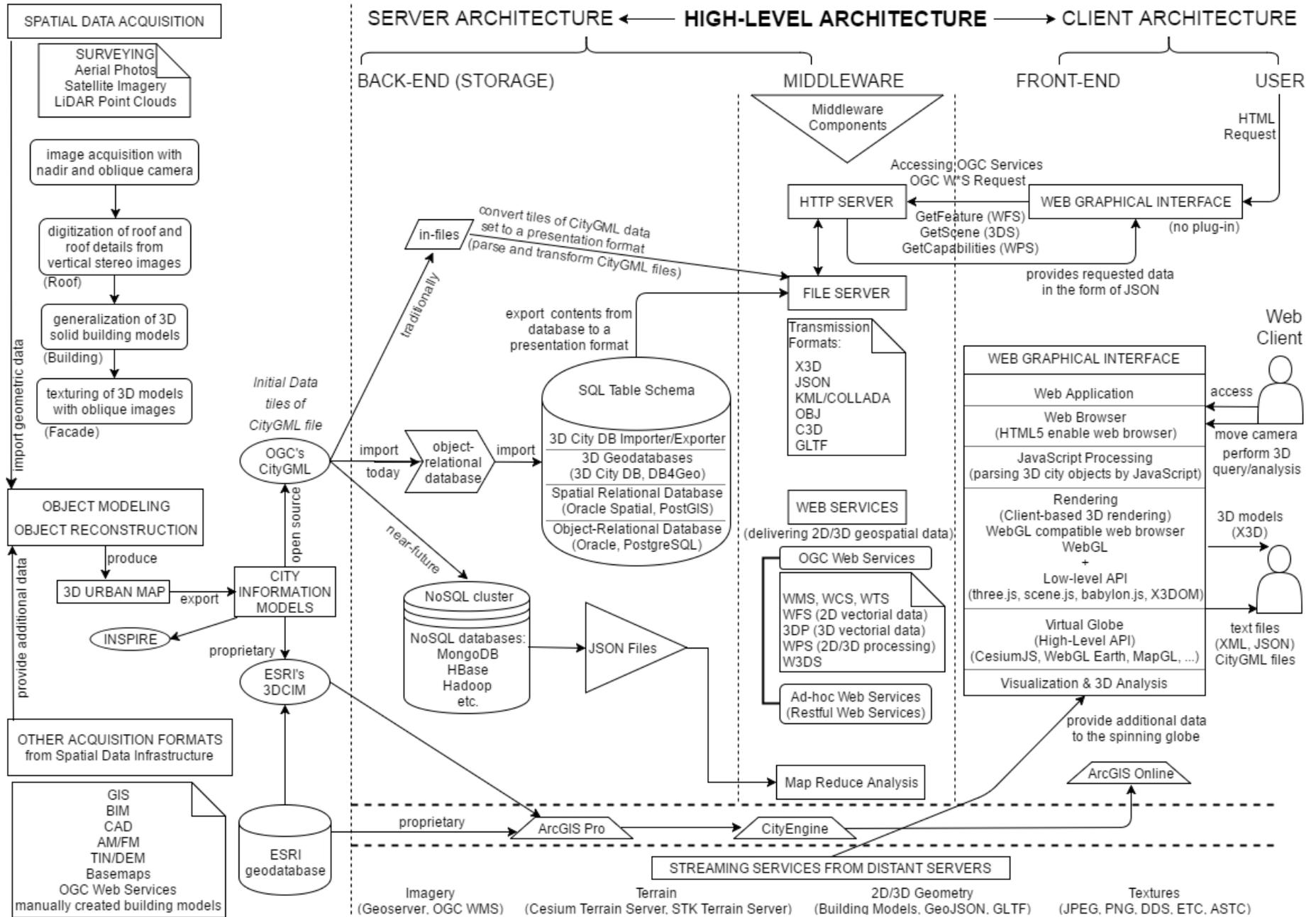
Figure 1. Three level architecture for the 3D geospatial applications on the web
