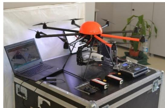
Figure 8. Octocopter with mounted hyperspectral camera
