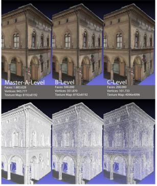
Figure 2: The three qualitative LoD defined according to different use of the 3D textured polygonal models – from urban and merely touristic web-based visualization to professional stand-alone 3D model editing and analysis with conservation, management and study purposes.
