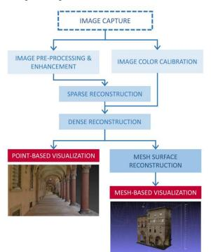
Figure 6: The photogrammetric pipeline for the 3D digitization and visualization of historical porticoes.
