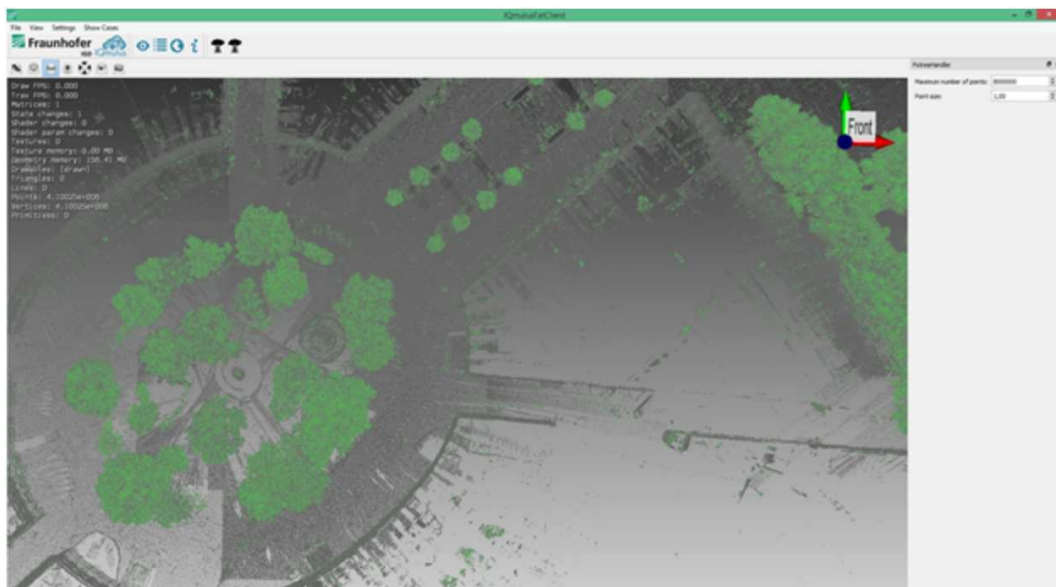
Figure 8. View on the Toulouse data set during asynchronous refinement. Note the difference in point density between the left and right parts of the image.
