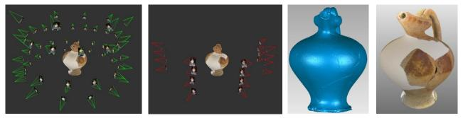
Figure 8: Imaging configuration for the ceramic jug: main imaging configuration without pattern projected onto the object (a); additional strips with images acquired with random pattern (b). Mesh model after the triangulation of the dense point cloud (c) and final textured 3D model (d).
