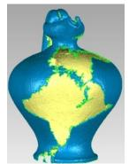
Figure 7: Reconstructed 3D model of the ceramic jug: the white textureless part was not reconstructed using a standard photographic equipment and photogrammetric approach.
