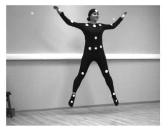
Figure 3. An actor with targets placed according BVH model
