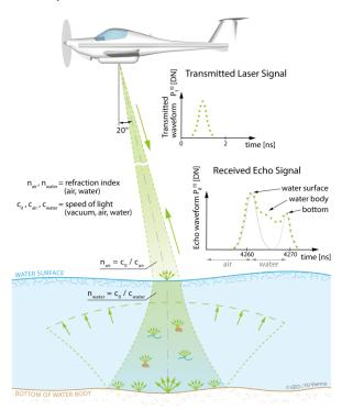
Figure 1. Diagram explaining ALB. See text for further information (©Department of Geodesy and Geoinformation Research Group Photogrammetry, E120.7).
