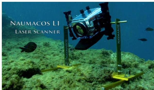
Fig. 8 - Portable scanning system, based on infrared laser light structured. When activated the system begins scanning rotating on its axis.
