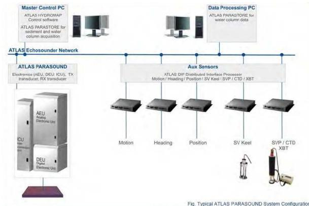
Figure 12. Parasound P – 35 Seismic system and subsystems
