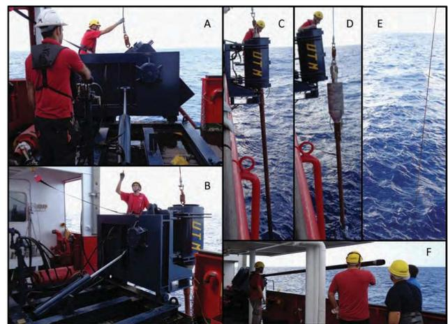
Figure 16. A and B - Detail cradle of gravity corer on the starboard deck; C, D and E - Launching the gravity corer; F - gravity corer on deck ready for extracting PVC jacket with the sedimentary record inside.
