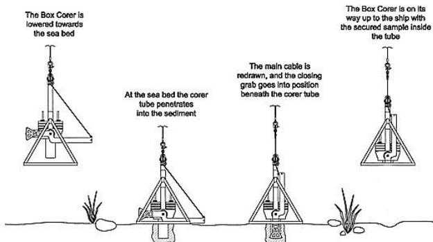
Figure 14. Detail of the box corer when it reaches the bottom.
