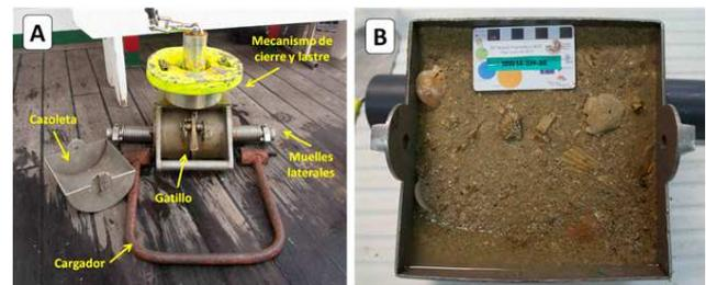
Figure 15. A) Shipek dredge with the different parts; B) surface sediment sample recovered in the bowl of the Shipek dredge.
