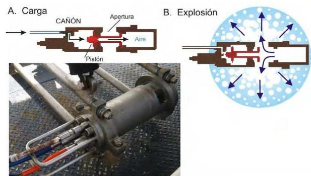
Figure 13. Photo detail of one of the guns and operation scheme.
