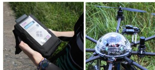
Figure 4. Measurement of illumination conditions using ASD spectrometer, Microtops sunphotometer and wideband irradiance sensor in the UAV.
