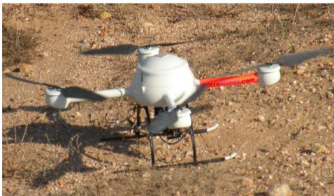
Figure 1. The vertical take off and landing UAV used for the flight mission
