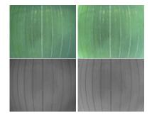
Figure 10: Two raw flight images (VIS+NIR) on the left and the corresponding vignetting corrected images on the right.
