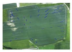
Figure 11: Orthophoto accuracy measurement with ground control points (red), corresponding RTK-GNSS measurements (yellow) and deviation vectors scaled by a factor of 10 (blue). The captured area is about  $550 \text{ m} \times 550 \text{ m}$ .
