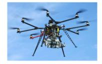
Figure 3: The camera system on board the Oktokopter.
