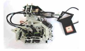
**Figure 2:** Close-up of constructed camera system with: (bottom) two board-level cameras in pan-tilt unit; (right) GNSS receiver mounted on top of the UAV during flight; (top) single-board-computer interfacing the cameras and the GNSS receiver.
