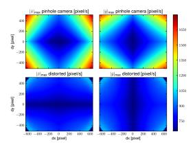
**Figure 6:** x and y pixel velocities under rotation of the camera (max. angular velocity) plotted against the pixel distance from the principal point. Results plotted for pinhole camera model (top) and distortion camera model (bottom).
