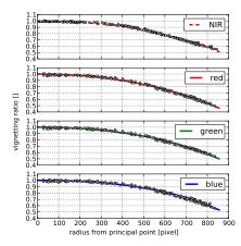
**Figure 8:** Results of calibration measurement series for each channel. Measurement points from the calibration images and fitted polynomial are plotted against radius from principal point (all data normalized).
