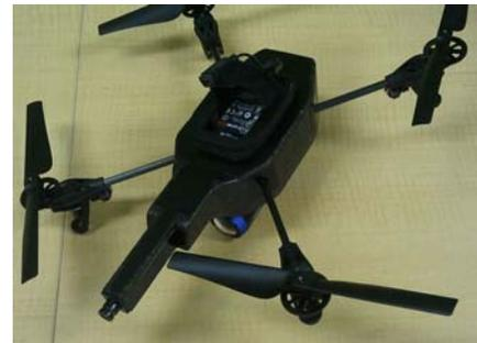
Figure 2. AR.Drone 2 UAV system with ION Air Pro camera.
